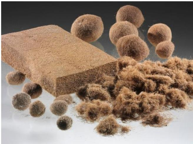
Neptune balls (a kind of seagrass) can be used as insulating material without the need for chemical additives.
