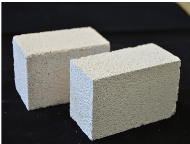
Aerated concrete made of brick (rear); aerated concrete made of sand-lime stones (front). © Fraunhofer IBP | Picture in color and printing quality: www.fraunhofer.de/en/press
