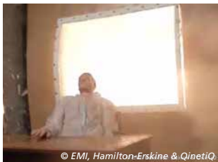
Fig. 9: Experimental full-scale investigation of the TecDur® BlastWall protection system. Left: Internal view during the test. Right: External view after the test.
